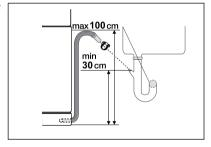
The sink plug must not be in place when the machine is draining as this could cause the water to syphon back into the machine.
